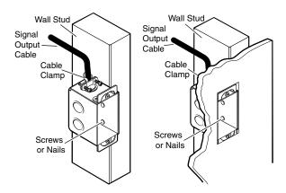
Figure 2-10 — Installing the wall box
